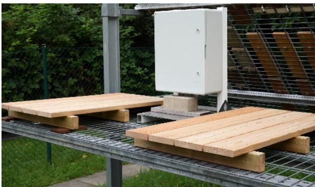
**Abb. 3:** Decking grates with 2 % (left) and 0 % (right) slope
